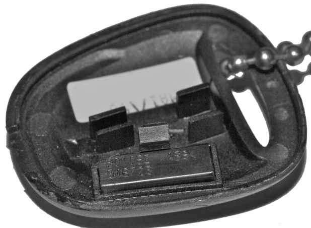
Figure 4: The Transponder is shown installed in the Key Head for Transponder Key 1. The installation is slightly different in the Key Head for Transponder Key 2.
