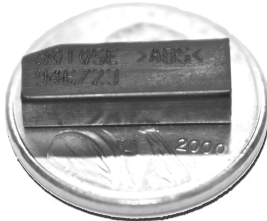
Figure 3: The Transponder is shown here resting on a US one cent coin. The transponder is 15mm in length. The transponder is not available as a separate spare part, only as part of the "Key Head" part for the Transponder Keys, and is integral with the "guts" of the Remote Keys.
