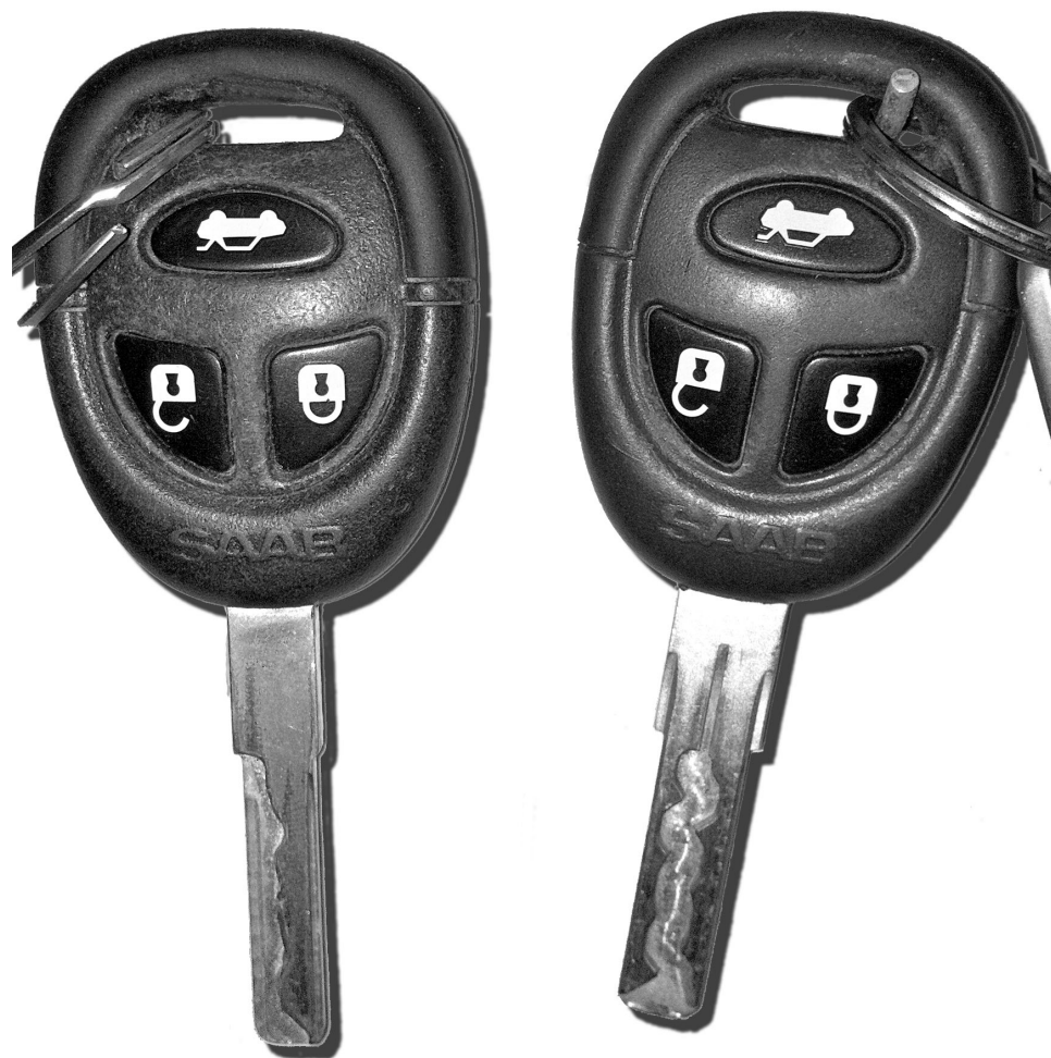
Figure 2: Detail of the two styles of "Remote Key". On the left, is "Remote Key 1". The blade is the same for this key, the two "Transponder Keys", and also the 9000 and 1994-1999 900. On the right, is "Remote Key 2", used on the 9-5 starting with chassis number 33026907 (late model year 2003). Although the "guts" that contain the transponder and remote lock & unlock are the same between the two keys, the key blades are different.
